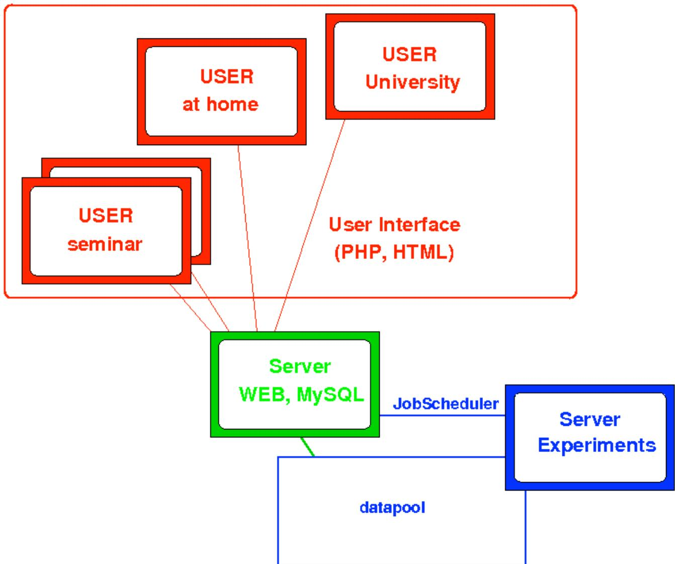
Figure 2: Components of the WEKUW system
